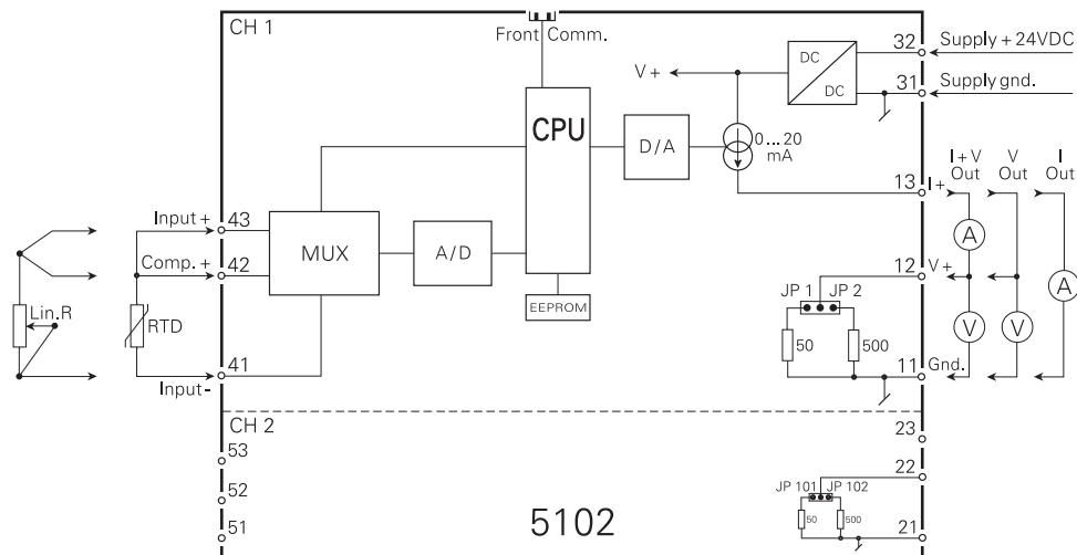
For 2-wire connection, short-circuit pin 42 and 43.
